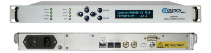
Figure 1-1. Digicast Media Router S2 Receiver – Front & Rear Panels
